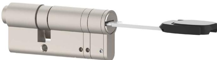
4. Adjust the internal side: if internal length of old cylinder is no more than 27.5mm, you do not need to do anything. If it is more than 27.5mm, please add the internal extensions together to form the difference between 27.5mm and your old cylinder internal length.
